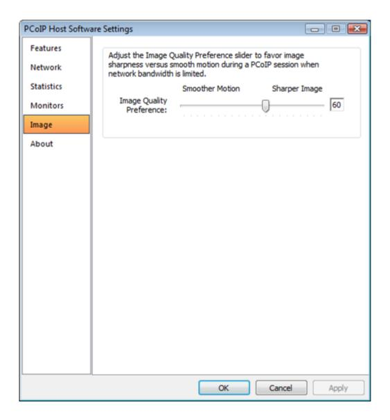
The PCoIP protocol adjusts image quality settings when the network connection between a PCoIP host and client is constrained and unable to provide enough bandwidth to support full frame rate video. The Image Quality Preference setting lets you configure a preference for smoother motion (higher frame rate) versus sharper image (higher image quality).
