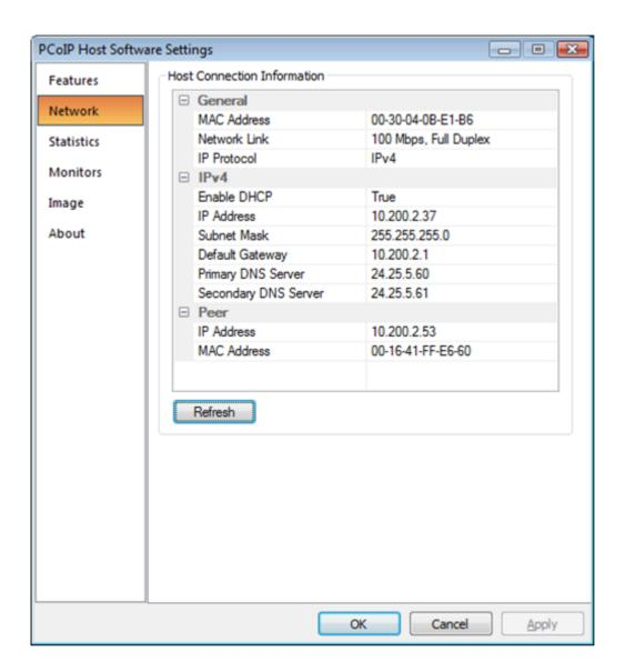
The *Network* tab shows the current network information for the host. This tab also reports status information on the NIC of the PCoIP host (speed, duplex setting, and link state – up/down). It also displays the IP and MAC addresses of the client connected to the host under the Peer settings.
